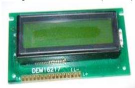
The HD 44780 is a liquid crystal dot matrix display Module that consists of LCD panel, LCD control driver, and driver and is capable of providing 16 characters x 2 lines display. It contains a controller, a data RAM and a character generator ROM required for providing display. Data interfacing is in 8-bit parallel or 4-bit parallel and data can be written in or read from a microprocessor.
