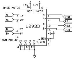
MCU cannot operate a dc motor directly. It operates the motor through the interfacing circuits. Here IC L293D acts as an interfacing unit between MCU and the DC motor.
